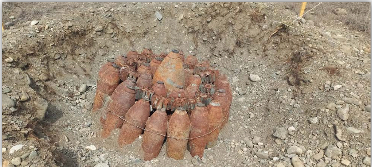
One of the recent discoveries in the liberated Aghdam district in Azerbaijan. Improvised trap mine containing one 240 mm 9M24F turbo jet rocket and more than thirty 120 mm mortar ammunitions (each containing 3 kg of explosives) placed together to maximize lethal power. Source: ANAMA, January 2023.
